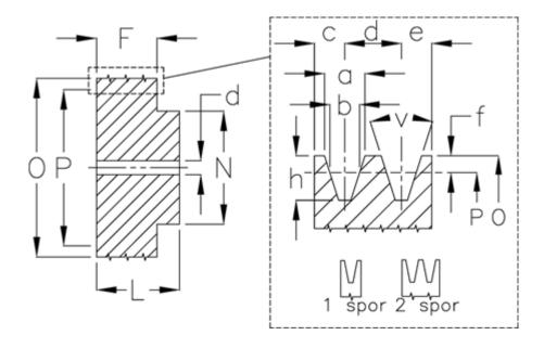
$\begin{array}{lll} d & = 10 \\ F & = 16 \\ L & = 28 \\ N & = 50 \\ Number of ribs = 1 \\ O & = 94.0 \\ P & = 90 \\ Type & = S \end{array}$
